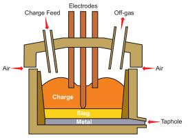
ARC Furnace cross section
