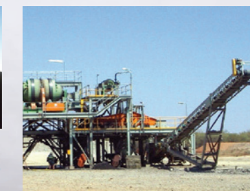
A typical mineral separation plant for upgrading manganese
